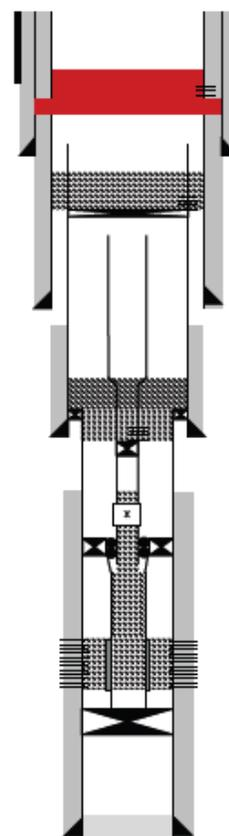
*Simplified Schematic Showing a ControlSEAL plug and squeeze*
